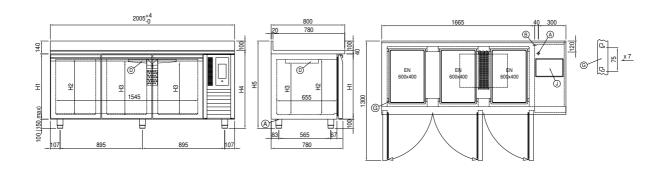
A: Power supply cable outlet B: Condensation water drain D: Airflow conveyor
