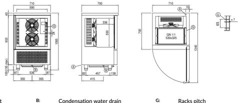
A: Power supply cable outlet B:
