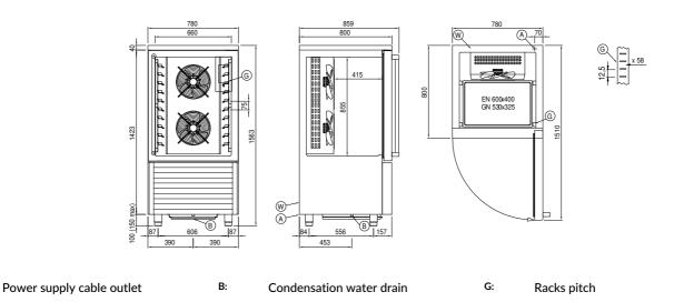
W: Water mains connection for humidifier - 3/4" female. Unloading not required
