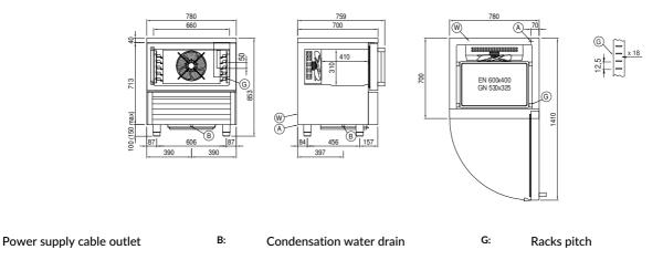
W: Water mains connection for humidifier - 3/4" female. Unloading not required
