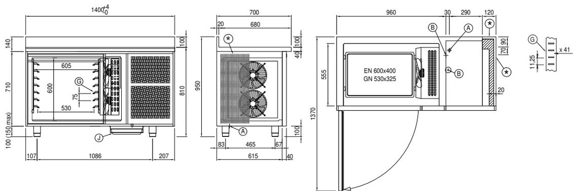
⊛ Foratura fianco, schiena e vano tecnico / Side, back and technical compartment drilling
