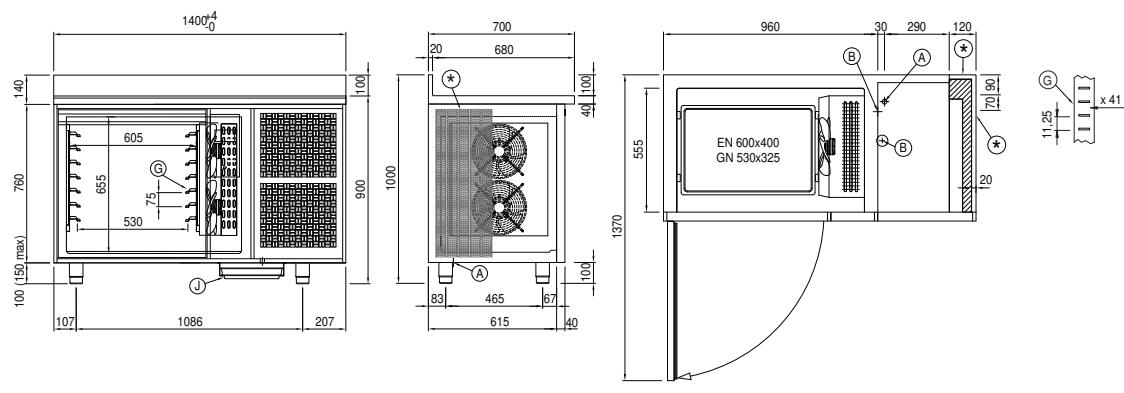
★ Foratura fianco, schiena e vano tecnico / Side, back and technical compartment drilling
