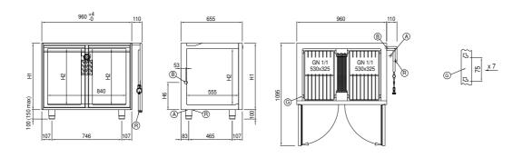
A: Power supply cable outlet B: Condensation water drain G: Racks pitch
