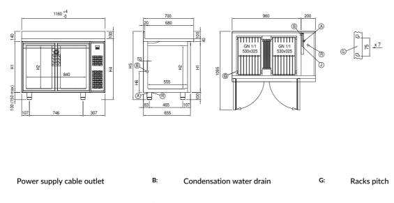
J: Automatic evaporation of R: Gas output pipes condensing water
