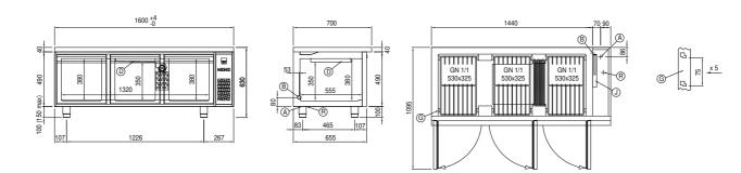
A: Power supply cable outlet B: Condensation water drain D: Airflow conveyor
