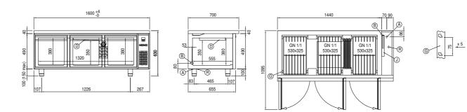
A: Power supply cable outlet B: Condensation water drain D: Airflow conveyor
