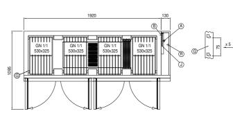
A: Power supply cable outlet B: Condensation water drain D: Airflow conveyor
