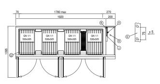
A: Power supply cable outlet B: Condensation water drain D: Airflow conveyor
