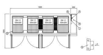
A: Power supply cable outlet B: Condensation water drain D: Airflow conveyor
