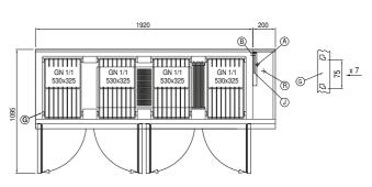
A: Power supply cable outlet B: Condensation water drain D:
