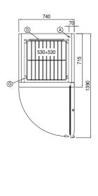
A: Power supply cable outlet D: Airflow conveyor G: Racks pitch
