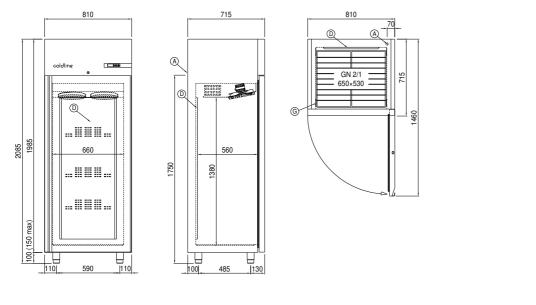
A: Power supply cable outlet D: Airflow conveyor G: Racks pitch
