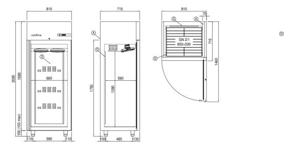
A: Power supply cable outlet D: Airflow conveyor G: Racks pitch
