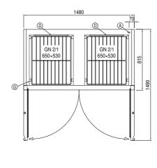
A: Power supply cable outlet D: Airflow conveyor G: Racks pitch
