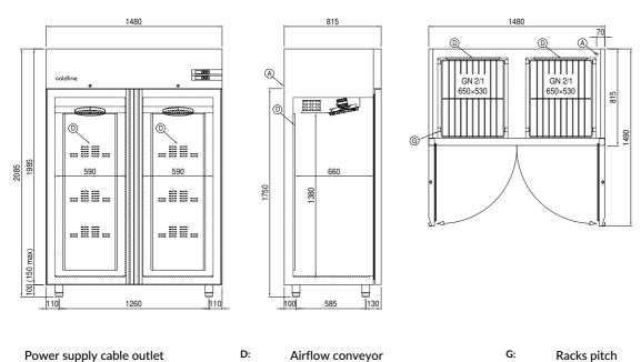
A: D: Power supply cable outlet Airflow conveyor
