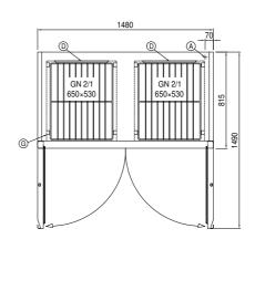
A: Power supply cable outlet D: Airflow conveyor G: Racks pitch
