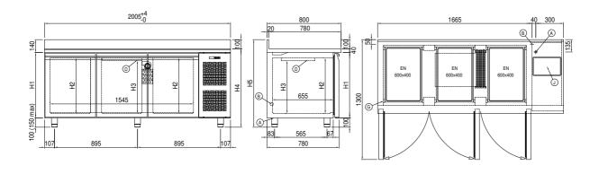
A: Power supply cable outlet B: Condensation water drain D: Airflow conveyor
