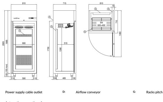
J: Automatic evaporation of condensing water
