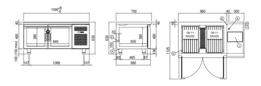
A: Power supply cable outlet B: Condensation water drain G: Racks pitch
