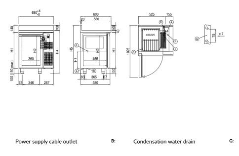
J: Automatic evaporation of R: Gas output pipes condensing water
