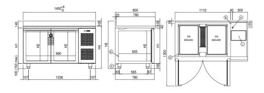
A: Power supply cable outlet B: Condensation water drain
