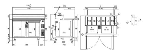
A: Power supply cable outlet B: Condensation water drain D: Airflow conveyor
