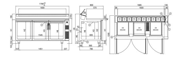
A: Power supply cable outlet B: Condensation water drain D: Airflow conveyor
