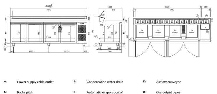
G: Racks pitch R: Gas output pipes
