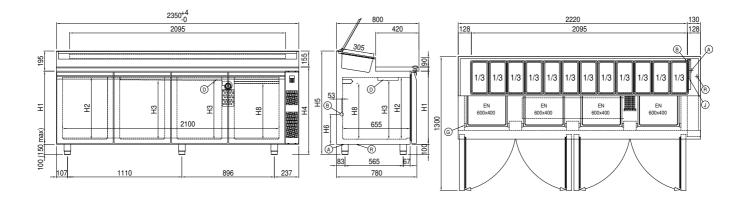
A: Power supply cable outlet B: Condensation water drain D: Airflow conveyor
