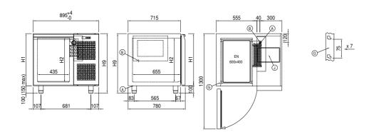
A: Power supply cable outlet B: Condensation water drain G: Racks pitch
