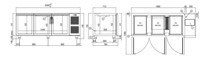
Power supply cable outlet B: Condensation water drain D: Airflow conveyor
