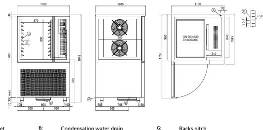
A: Power supply cable outlet B:
