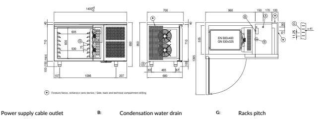
J: Automatic evaporation of condensing water
