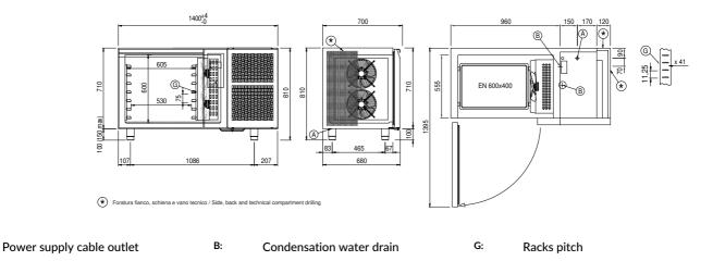
W1: Water inlet/outlet for condensing unit - 3/4" male
