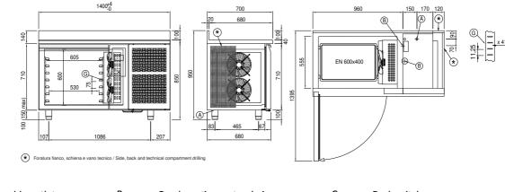
A: Power supply cable outlet B: Condensation water drain G: Racks pitch
