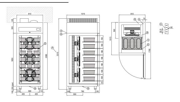
A: Power supply cable outlet B: Condensation water drain G:
