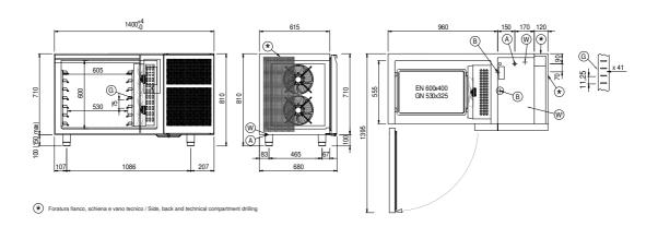
A: Power supply cable outlet B: Condensation water drain G: Racks pitch
