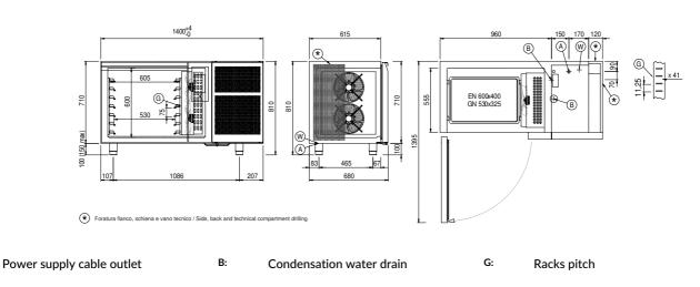
W: Water mains connection for humidifier - 3/4" female. Unloading not required
